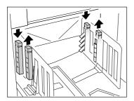
Press to open the two Paper Arrangers (right and left) closer to the machine.
