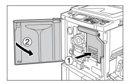
Return the Master Making Unit to its original position and close the Front Cover.
