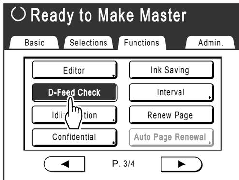
The button changes from being highlighted (b/w) to the normal display, and “D-Feed Check” is set to “OFF”.
