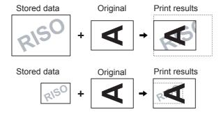
The storage data is overlaid after being centered at the top of the original. You cannot adjust the overlay position.
