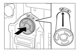
Align the arrow on the Ink Cartridge to the  $\ lacktriangledown$ mark on the print drum (cylinder) unit, and insert until it stops.
