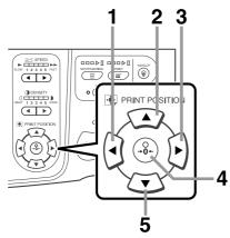
Each press shifts the print position downward in steps of about 0.5 mm (1/64").
