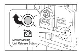
If the indicator is off, press the Master Making Unit Release Button to turn it on.
