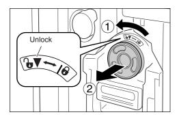
Turn the Ink Cartridge to the counter clockwise ('b) and then pull it out.
