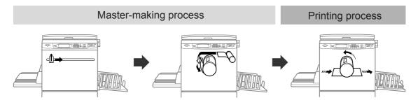
A placed original is scanned by the scanner, and a generated master is rolled around the Print Drum (Cylinder). After a while, proof copy is performed. After checking the print result, enter the number of copies to be printed and start printing.
