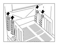
Press to open the two Paper Arrangers on the more heavily printed side.
