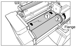
Insert the leading edge of the master into its entrance under the Master Guide Flap and advance it as far in as it will go ( 1). If the Master is loose, turn the flange at the right towards the rear and rewind (2).
