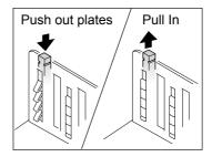
Alignment of paper is affected by sizes and strength of paper. Adjust the Paper Arrangers so that printed paper is aligned.
