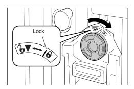
Turn the Ink Cartridge clockwise ( ) and lock in position.
