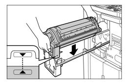
Align the ▼ mark on the Print Drum (Cylinder) with the **A** mark on the guide, and place the Print Drum (Cylinder) horizontally onto the guide.
