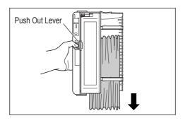
Tilt the Master Disposal Box forward and directly discard the used master into the garbage box (or bag) by grasping the Push Out Lever.
