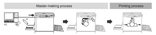
Transfer the original data created with a computer to the machine via a network or USB Flash Drive. A generated master is rolled around the Print Drum (Cylinder).
